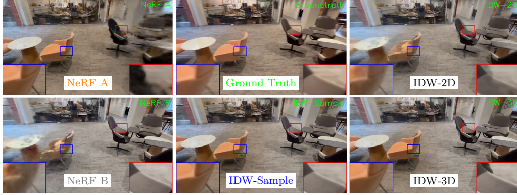
Figure 2.6: Qualitative comparison of NeRF blending methods. While individual NeRFs and baseline blending methods (IDW-2D, IDW-3D) struggle to reconstruct both chairs clearly, our proposed IDW-Sample method produces a sharp, high-quality rendering that successfully integrates the best information from both sources.
