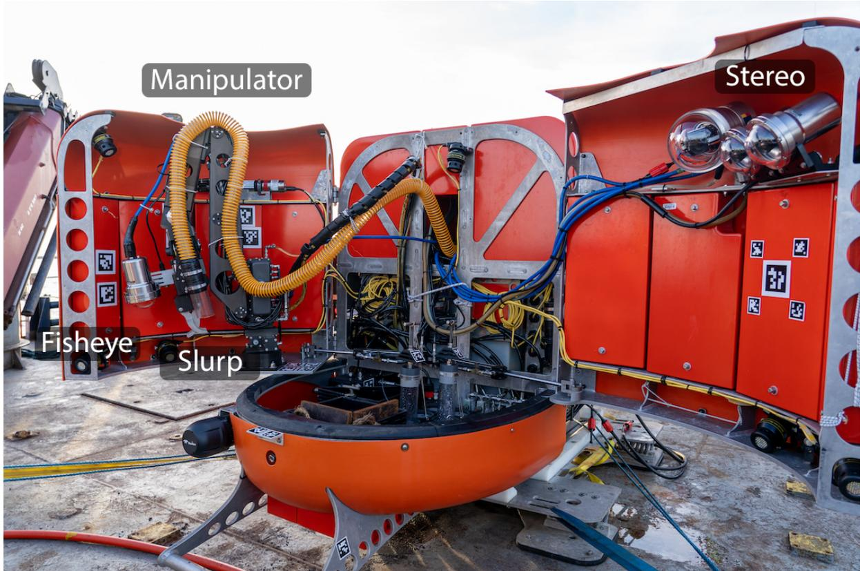
Figure 14: The *NUI* vehicle is outfitted with clam shell doors that can be closed to reduce drag when cruising and opened to perform manipulation tasks. The manipulator is mounted to the starboard door and the stereo cameras are mounted to the port door.
