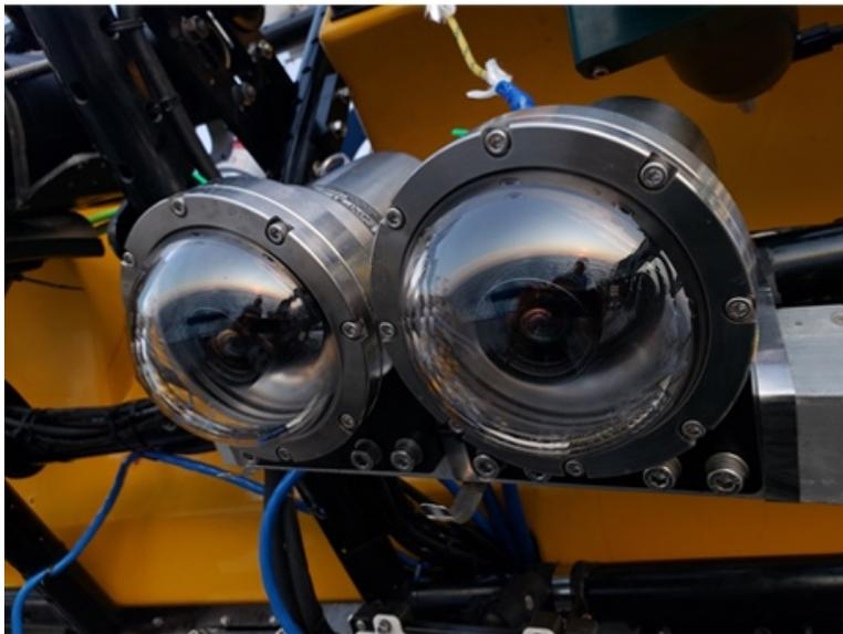
(b) Vehicle-mounted stereo camera
