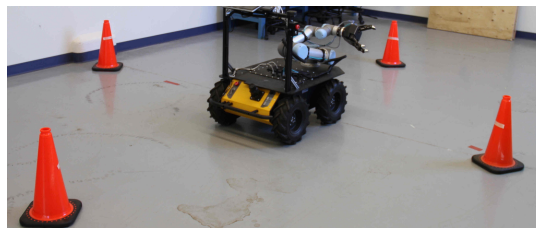
Fig. 4. An illustration of the experimental setup for the modified Clearpath Robotics Husky A200 mobile robot. Each of the four cones represented an object with the semantic tags “Building”, “Traffic Cone”, “Traffic Barrel”, and “Car”.
